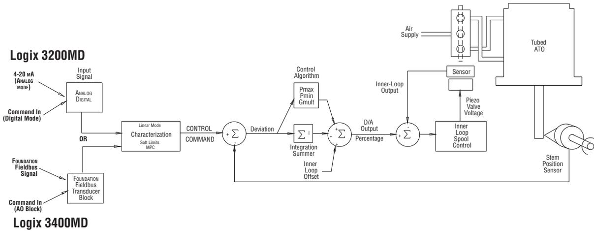
Figure 1: Logix 3000 Series Digital Positioners Schematic (air-to-open configuration)
