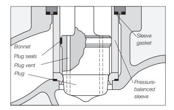
Flow direction is under-the-plug for fail-closed and over-the-plug for fail-open. The seal area less the stem area is designed to be slightly larger than the seat area; therefore, the plug is off-balanced to close for flow under the seat and off-balanced to open for flow over the seat.
