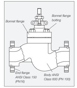
Figure 7: Separable end and bonnet flanges
