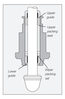
3. Two widely spaced stem guides, when used with the Mark One valve's large plug stem diameter, provide exceptional guiding. The upper stem guide also acts as a packing follower; the lower guide is situated close to the plug head for additional guiding support, ensuring accurate alignment of plug and seat ring.
