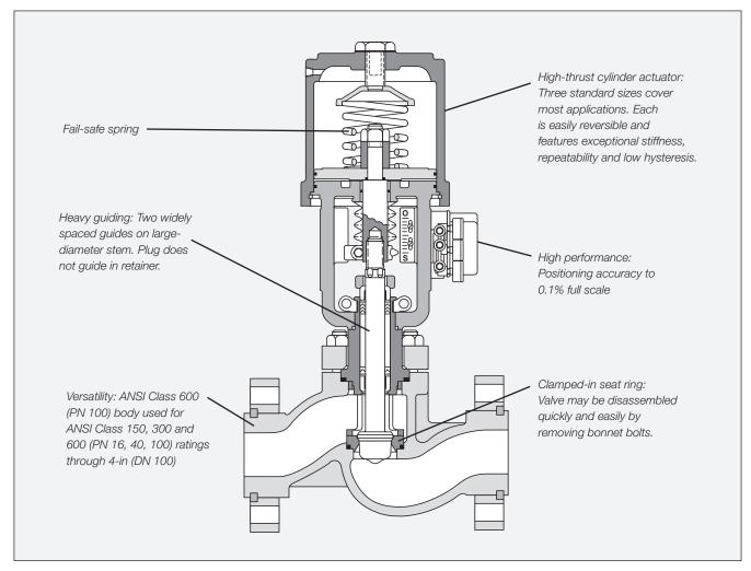
Figure 1: Valtek Mark One globe control valve
