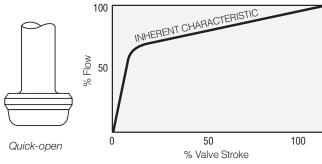
Figure 13: Flow characteristics
